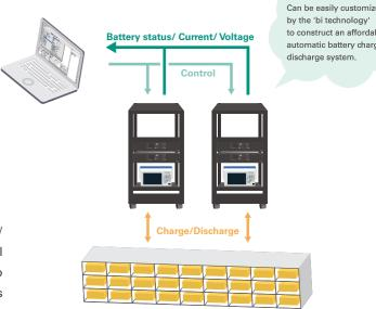
the charge or discharge commands to be sent to the biATLAS depending on the battery status, the biATLAS can offer even the current and voltage information for charge and discharge.
