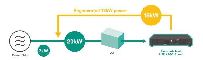
Furthermore, by the connection of the biATLAS-D525 Load to the power distribution panel common to the power supply equippment for an evaluation and inspection system, the regenerated energy can be used by the power supply equippment again, and the evaluation and inspection system in an energy circulation type can be constructed. The device under target with large capacity can be evaluated at only low power from the power grid.
