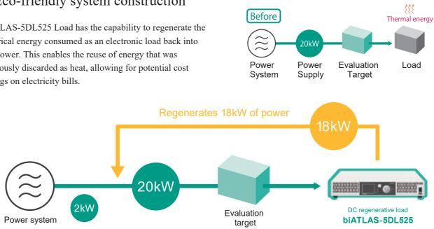
Furthermore, by connecting the biATLAS-5DL525 Load to the common distribution board of the evaluation and testing system's power supply, the regenerated energy can be reused by the power supply unit. This allows for the construction of an energy-circulating evaluation and testing system, enabling the evaluation of large-capacity devices with minimal power from the power system.
